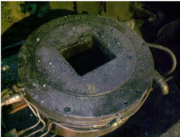
Steel Casting Mold made from Copper.
