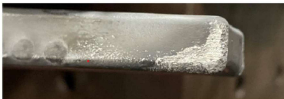
Example of soldering on a core pin after a production die casting run (photo courtesy of Mercury Marine). This buildup tears the casting at ejection and may result in dimensional and leaking defects.
