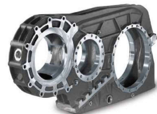
ICE II gearbox housing artificially aged Sand casting 1800 × 850 × 250 mm, weight: 175 kg: AlCu4Ti
