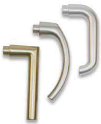
Door handle Gravity die casting, decoratively anodized 135 × 65 × 15 mm, weight: 140 g: AIMg3
