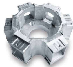
Cast node for glass dome design Gravity die casting Ø 260 × 110 mm, weight: 2.3 kg: AlZn3Mg3Cr
