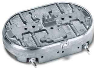
Heating plate for espresso machine High pressure die casting, flanged 138 × 91 × 42 mm, weight: 0.71 kg: AISI9
