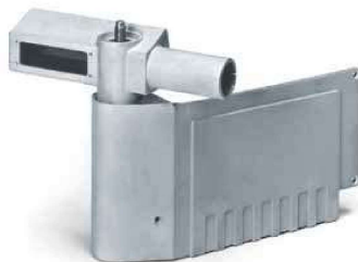
Input housing for autopilot on offshore yachts Sand casting, anodically oxidised 290 × 210 × 40 mm, weight: 0.4 kg: AIMg5
