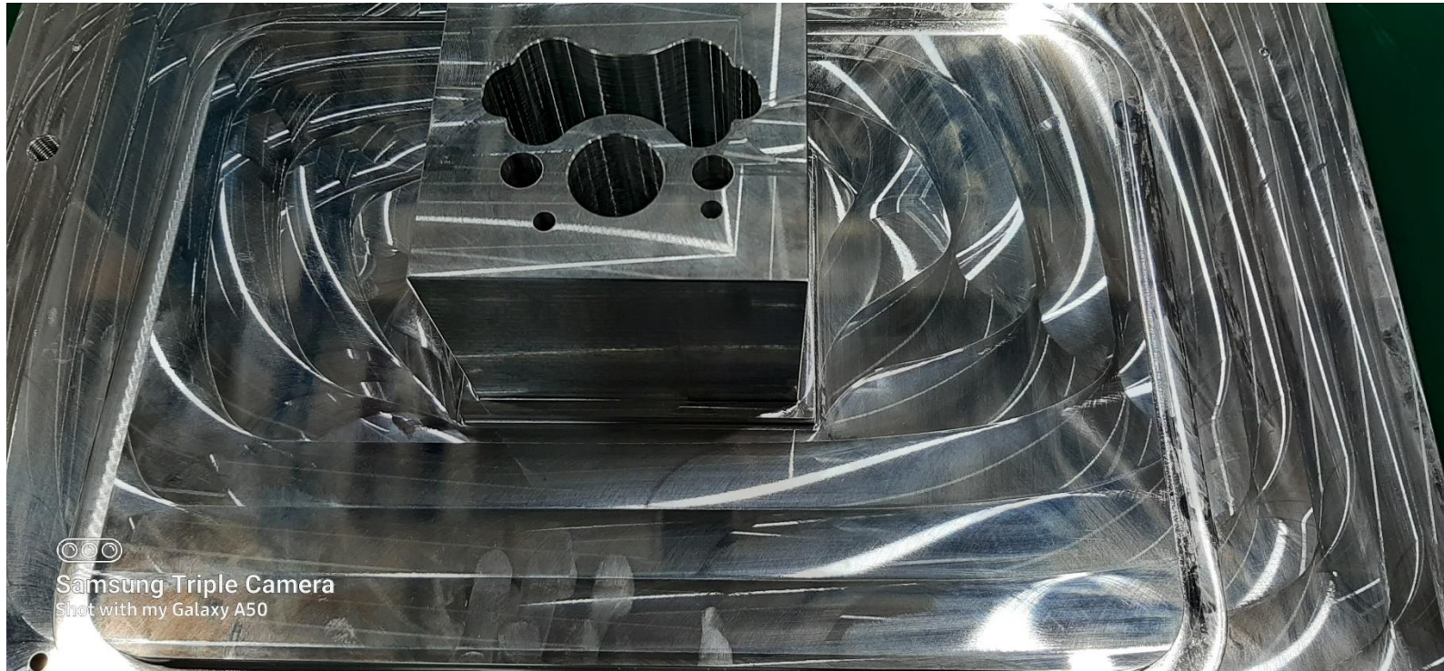
Index 3 – No water StAIN mark on aluminium jig
