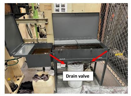
3. The workpiece should be dipped in rust-preventive oil once to clean dirt and once to coat the rust-preventive oil on the workpiece.
