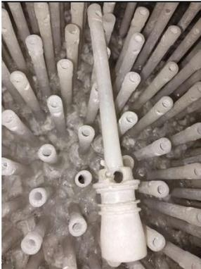
1. Picture of nozzle inside freezer machine. Material made from nylon.
