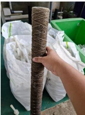
4. Picture of filter for intake water for freezer machine.
